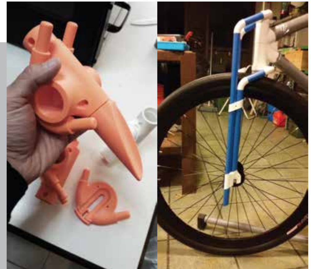
assembling joints, with screws and epoxy glue
