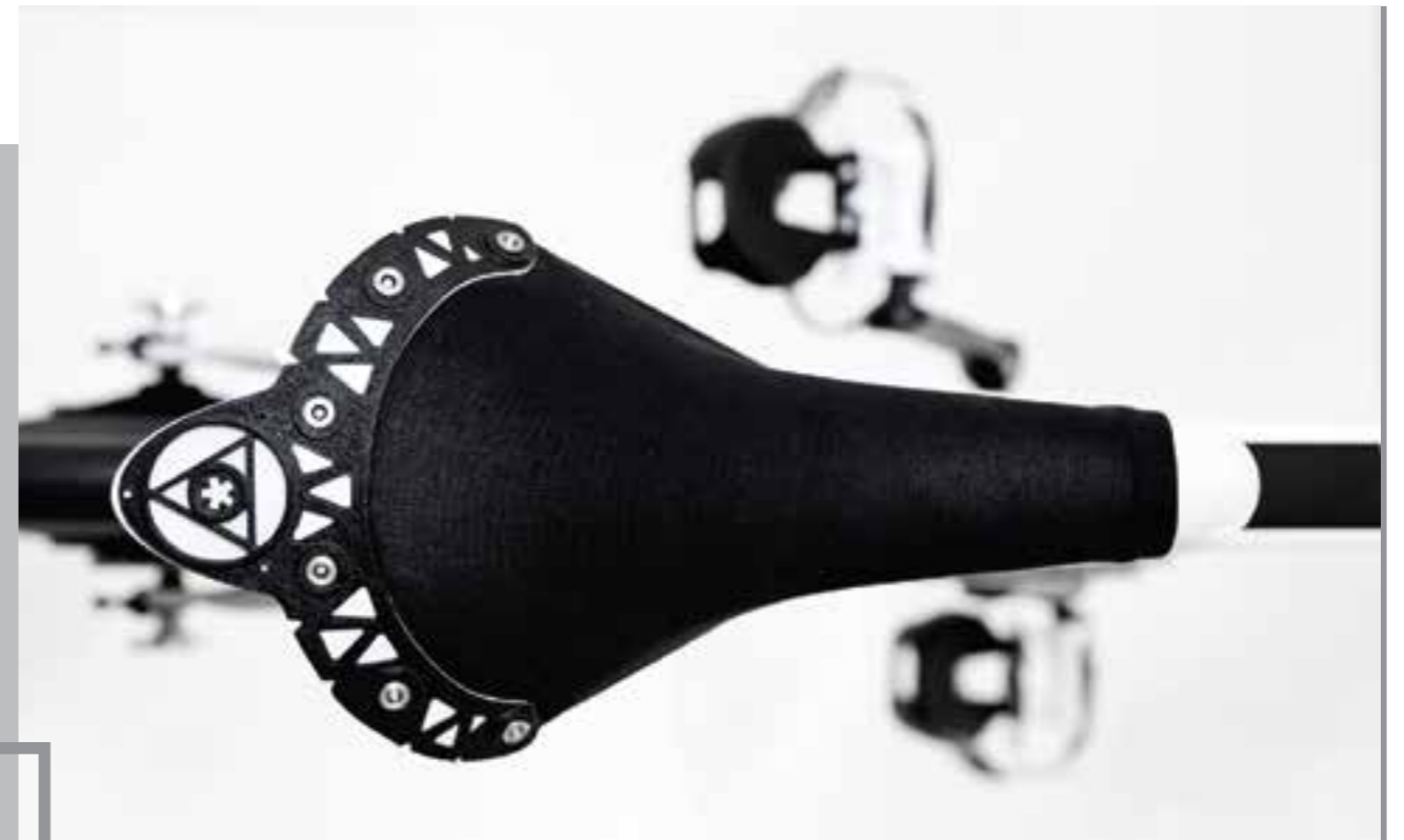
the back of the saddle hides a led light activated by movement
