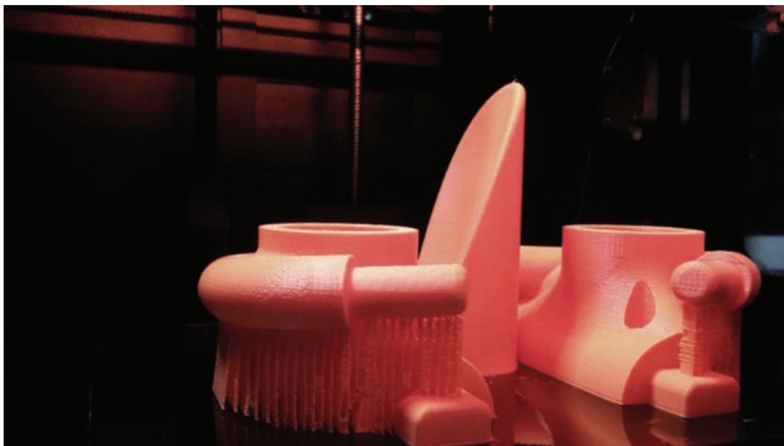
Printed Bottom Bracket/seat Tube ( this frame is double simmetrycal !)
