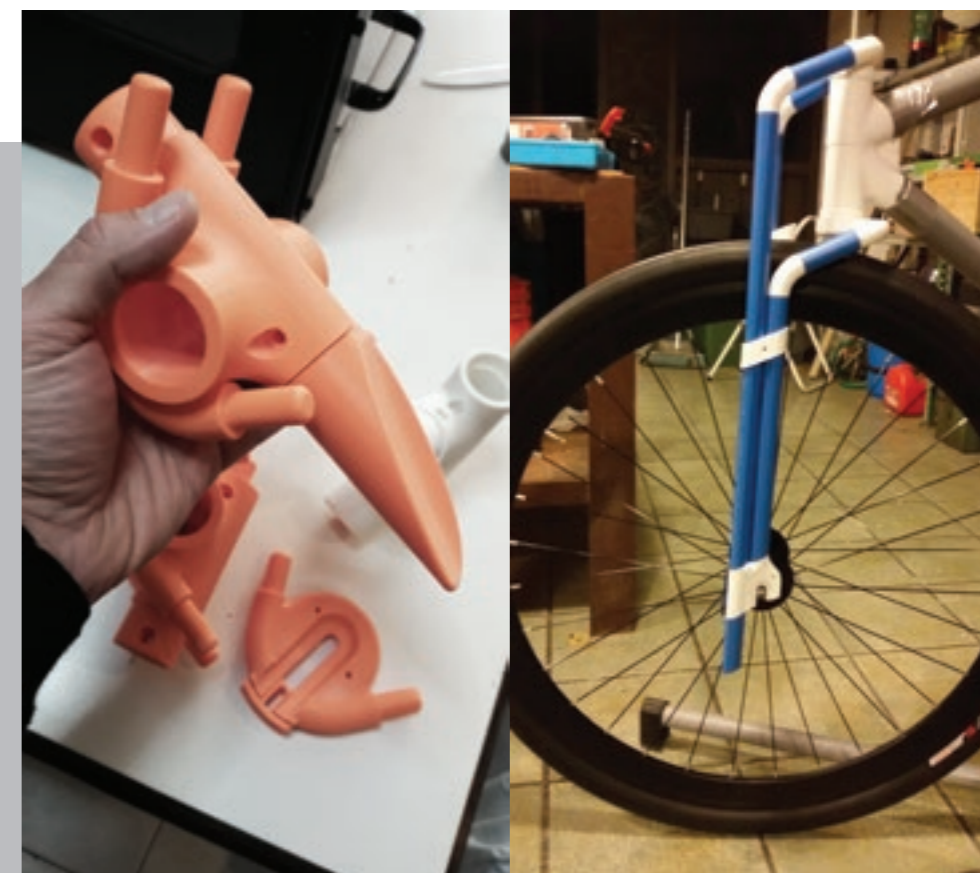
assembling joints, with screws and epoxy glue
