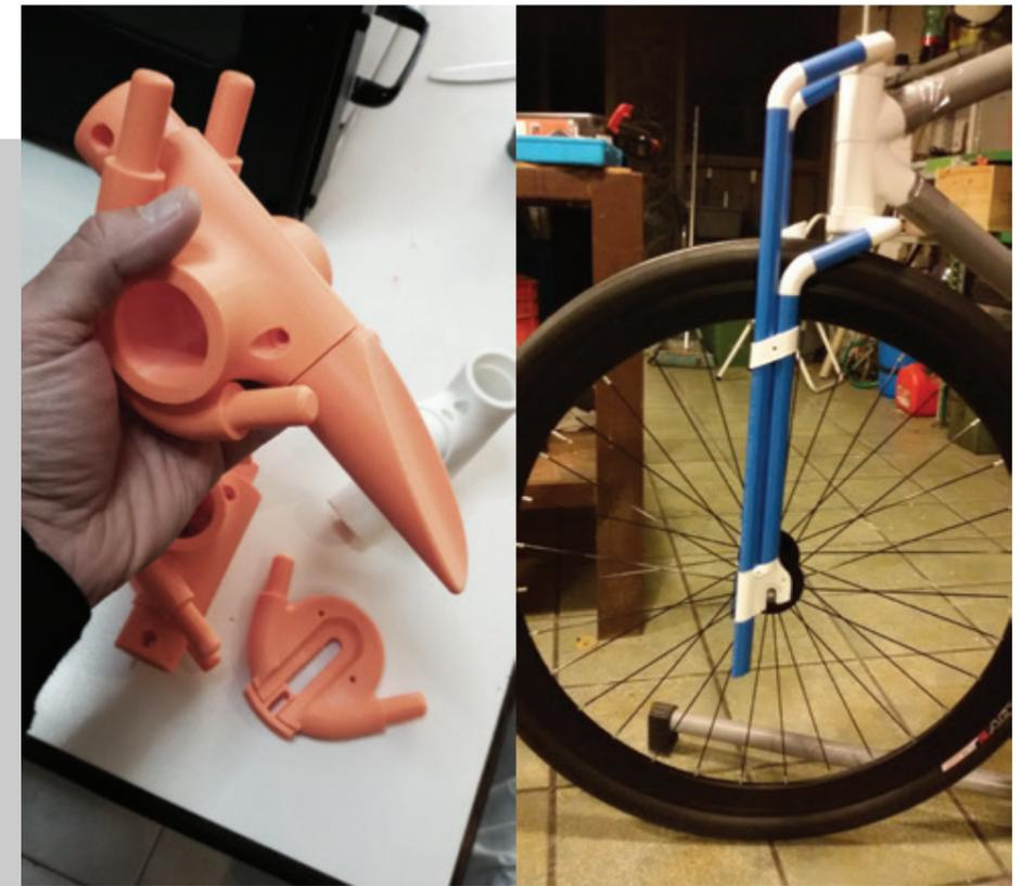
assembling joints, with screws and epoxy glue
