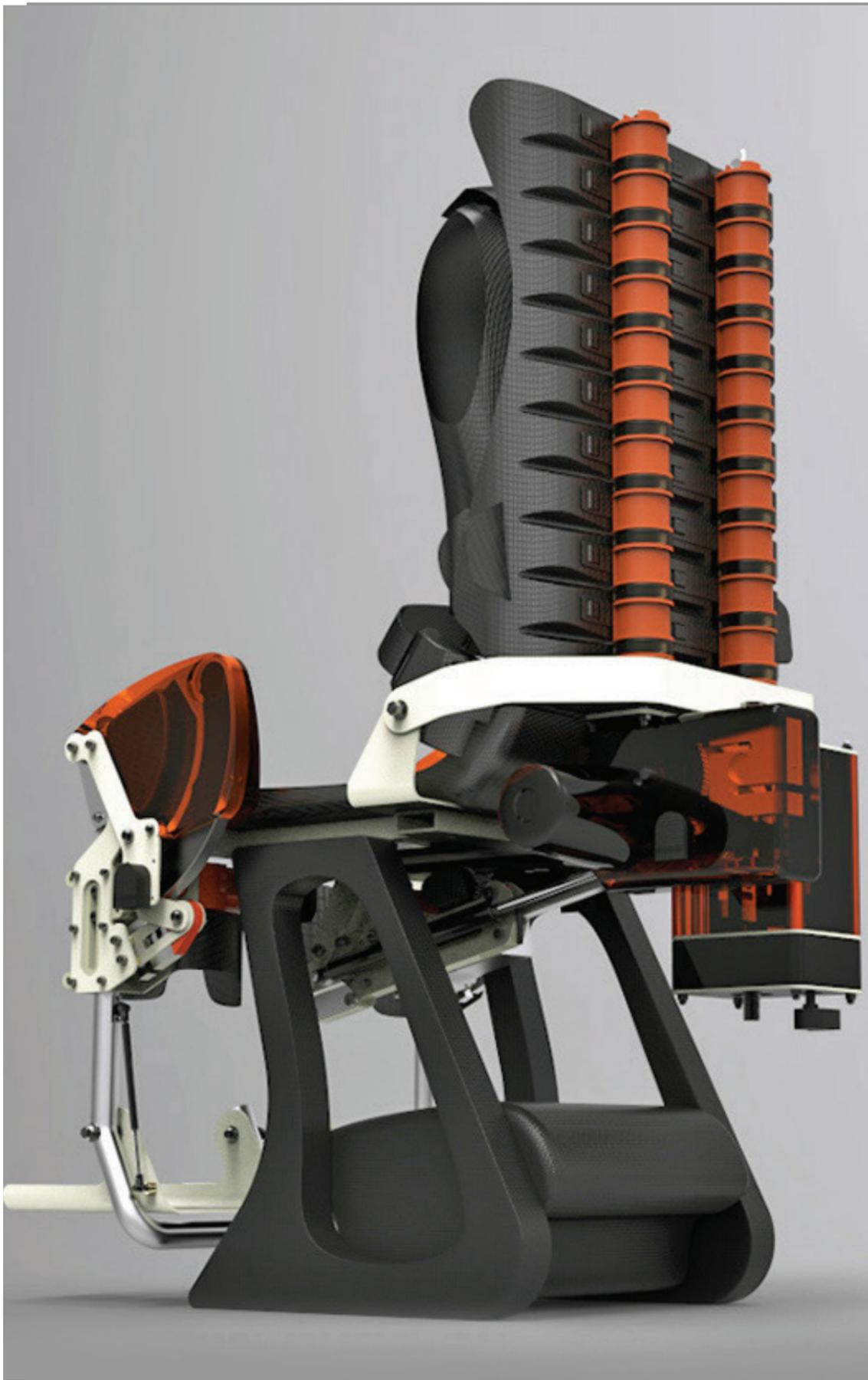
SACE 2 is a robot, an exoskeleton, connected to the human Body it can restrict or help the movements. Even the artificial spine can flex through a cable system
